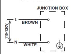
A standard 120-volt power cord (field supplied) provides the electrical connection. The unit is designed to operate on a separate 20-amp circuit.
